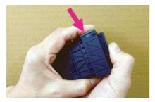
② While pushing the ECU, push the gray lever back to its original position. At this time, the ECU is linked to the movement of the gray lever The system goes deeper and is set in the correct position.
