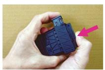
① Check the orientation of the ECU, insert it slowly. If you mistake on the front and back, can not insert the coupler slot.
