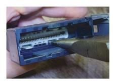
Using radio pliers or similar tools, pull horizontally and gradually so as not to damage the wide claws that protrude from four locations on the top, bottom, left, and right sides of the white part at the back inside the coupler slot. Once the terminal looks like the "correct example", do not pull it any further.
