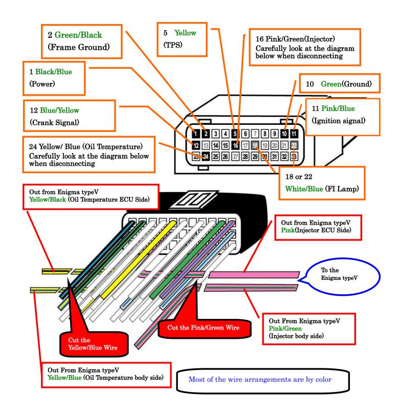
ECU terminal connected 9wires 1,2,5,10,11,12,16,18or22,24. Please confirm the picture.
