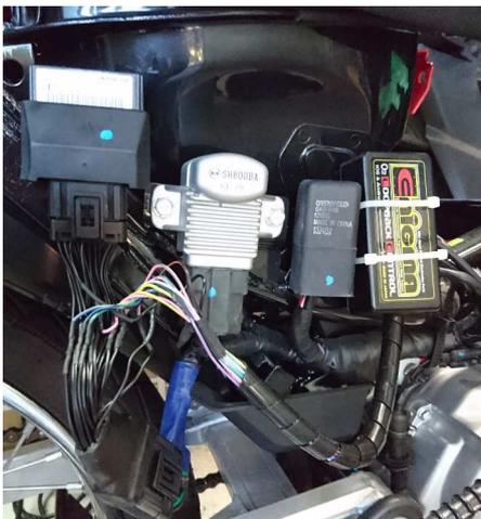
Remove the coupler connected to the ECU, process the wiring and interrupt ENIGMA.
