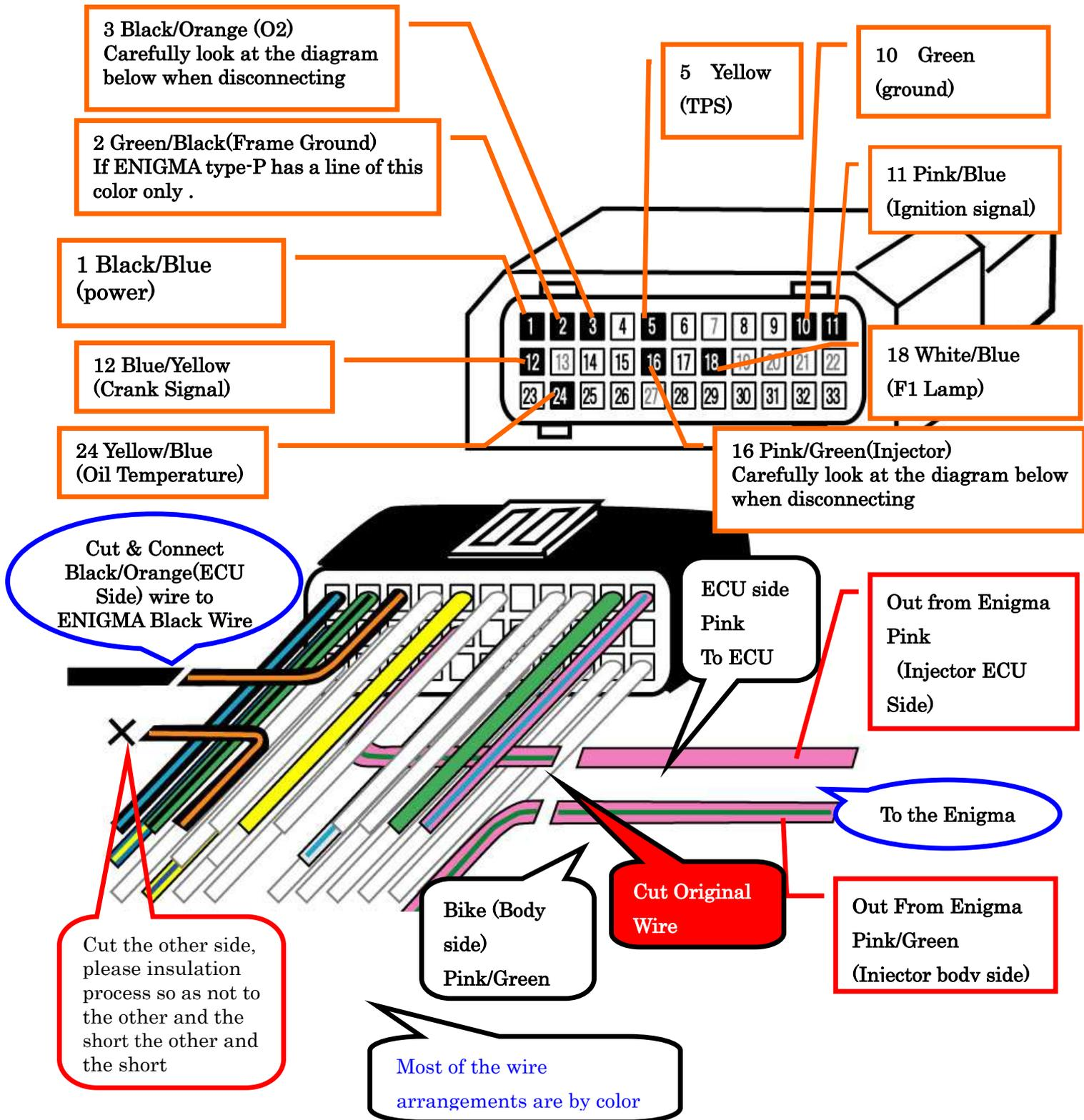
ECU terminal connected 10wires 1, 2, 3, 5, 10, 11, 12, 16, 18, 24. Please confirm the picture.
