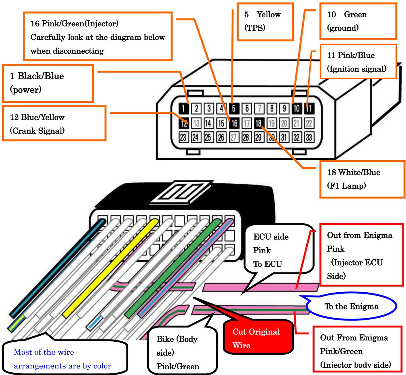
ECU terminal connected 7wires 1,5,10,11,12,16,18.Please confirm the picture.
