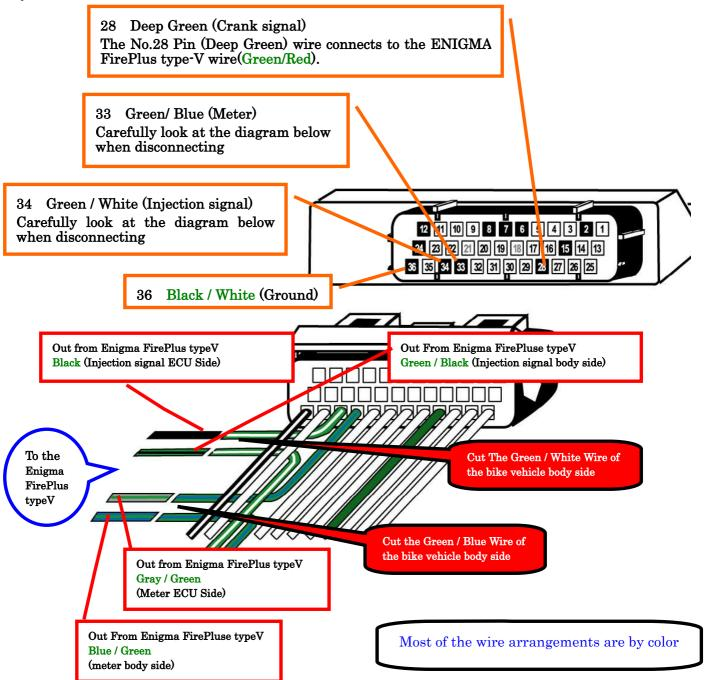
ECU terminal connected 11wires 2, 6, 7, 8, 12, 15, 24, 28, 33, 34, 36. Please confirm the picture.
