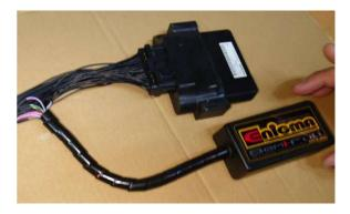
Disconnect the ECU from the body coupler and connect the ENIGMA coupler between the ECU and the body coupler. Attach the ECU to the ENIGMA coupler.
