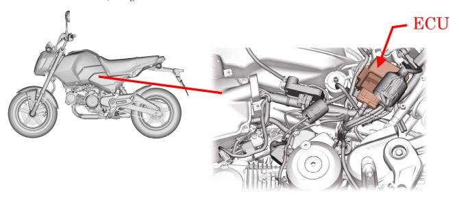
After removing the ECU to the rubber mount, disconnect the ECU from the body coupler and connect the ENIGMA SemiFull coupler between the ECU and the body coupler.
