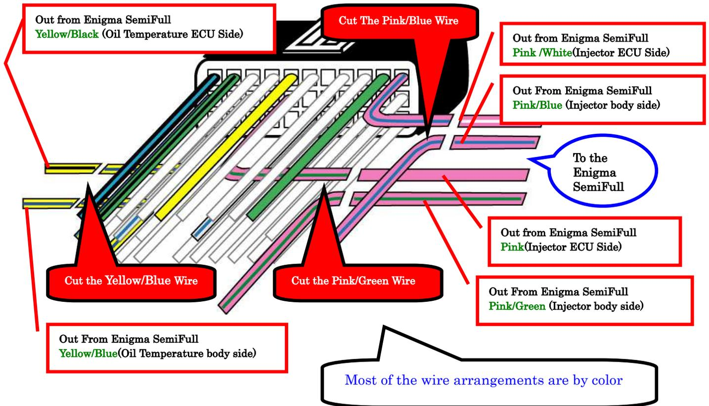
ECU terminal connected 10wires 1, 2, 5, 10, 11, 12, 14, 16, 18, 24. Please confirm the picture.
